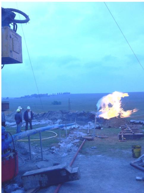
Safely flaring gas from Stage 1 of pilot production well KA-03PT 21<sup>st</sup> November 2012
