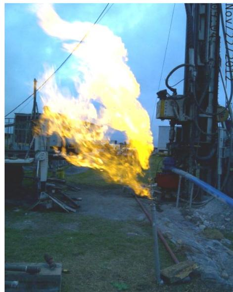
**Safely flaring gas from Stage 1 of pilot production well KA-03PT
