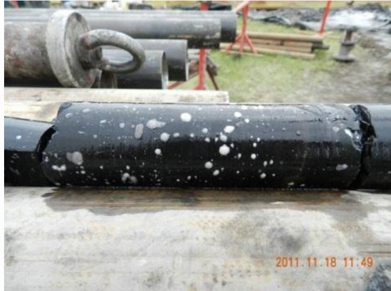
Figure 3. KA-02 Gassy coal sample (311m) prior to containment in a canister
