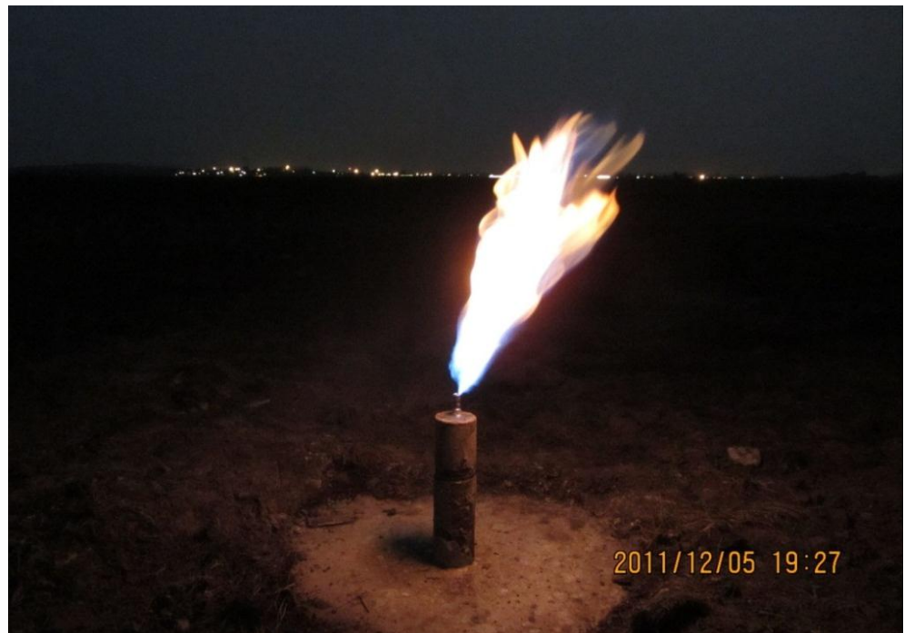
Figure 1. Drill hole KA-06, controlled flaring of spontaneous gas flows.
